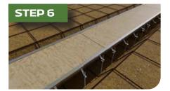
Use plywood or equivalent to replace the grating on the drain during the installation stage. This will ensure no concrete is spilled into the drain, and will eliminate damage to the drain due to the concrete expansion.
