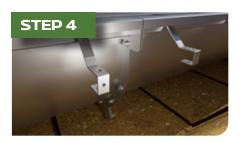
After the silicone bead has been applied, secure the drain connections by tightening the nuts and bolts at flanges.
