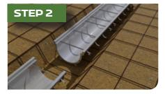
Bolt all sections of the trench drain together using the numbered flanges as a guide. For example, if you have the drain 102, 203, 304 and a catch basin: First, bolt flange 4 of drain 304, which is the deepest section, to the catch basin flange. Next, bolt flange 3 of drain 304 to flange 3 of drain 203. Finally, bolt flange 2 of drain 203 to flange 2 of drain 102.
