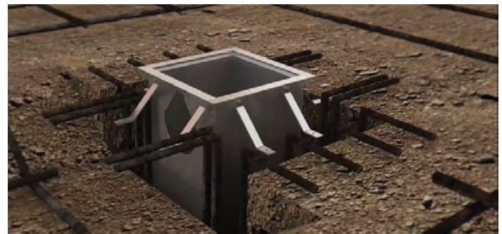
PIPE CONNECTION TO THE CATCH BASIN OUTLET
