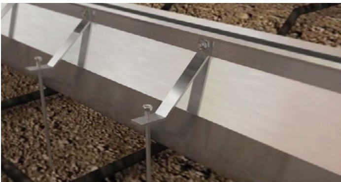
THREADED ROD CONNECTION BETWEEN LEVELING BRACKET AND THE CONCRETE BASE
